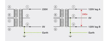
effect, means that they will give you a 240 volt single phase supply. For these applications we offer transformers with a 'European' output (230 volt live and neutral) and a 'USA' output (two legs of 120 volt and a neutral - also referred to as a 120-0-120 or a 120 / 240 type supply. A 240 volt supply is normally available at either 50 amps (12 kW) or 100 amps (24 kW).
